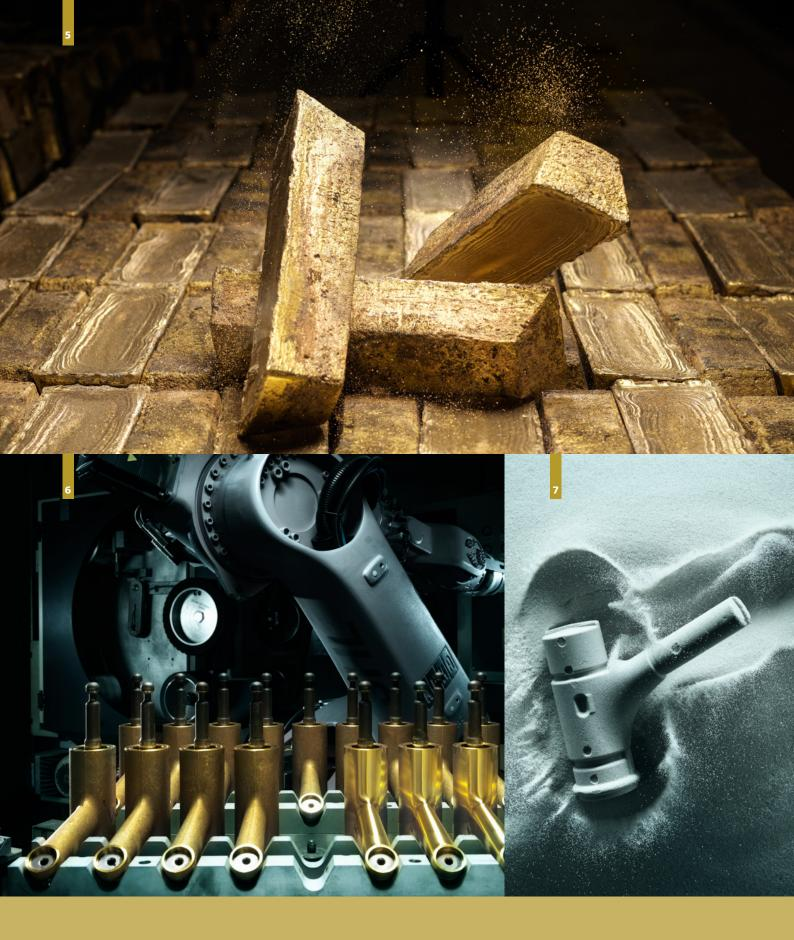
5 — To make the fittings, pure brass, which arrives in the form of ingots, is used. 6 — The basic shape of the fitting in brass. 7 — With low-pressure die casting, the brass is first melted and then poured into sand molds, creating the basic shape of the fitting in brass.
