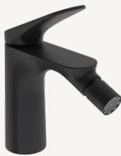
3743226333 Bidet faucet | Flexible pipes | Pop-up waste | Connection size: G3/8 | Projection: 127 mm
